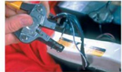
P14-4 Using the correct size stripper, remove about  $\frac{1}{8}$  inch of the insulation from both wires.
