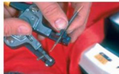
P14-5 Now remove about  $\frac{1}{8}$  inch of the insulation from both ends of the replacement wire. The length of the replacement wire should be slightly longer than the length of the wire removed.
