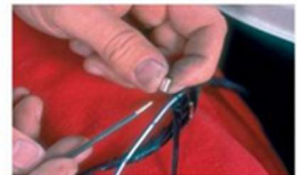
P14-6 Select the proper size splice clip to hold the splice.
